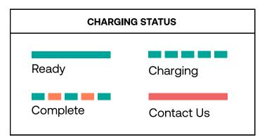
Vehicle will automatically stop charging when it is fully charged.
